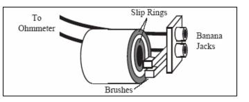
soldered to the copper slip rings (Fig. 2) on the side of the cylinder. The brushes provide an electrical connection between the slip rings and the banana plug connectors. By plugging an ohmmeter into these connectors, the resistance of the thermistor, and therefore it's temperature, can be monitored, even when the cylinder is turning.
